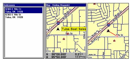
Address search result list (left). Map Page showing location of the address on the map (center) highlighted by cursor. After the address is located, you can navigate to it ("D" symbol for destination) (right).
